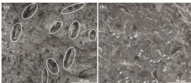
Fig. 1. Dispersion states of GNPs in the two polymers: SEM images of (a) PLA and (b) PBAT nanocomposites with 3wt% GNPs.
