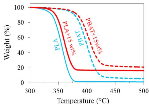
Fig. 4. TGA curves of pure PLA and PBAT and their 15wt% GNP nanocomposites.
