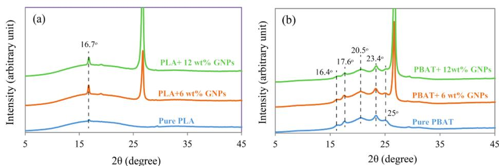
Fig. 2. X-ray diffraction patterns of (a) PLA and (b) PBAT nanocomposites.
