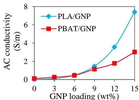
Fig. 3. AC conductivity vs. GNP loading at 10 GHz.
