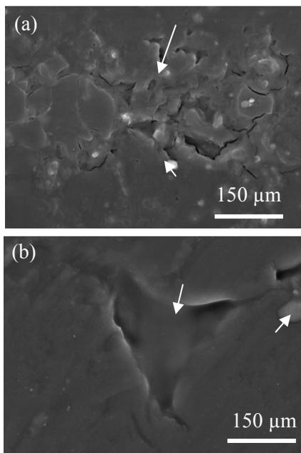
Fig.3. SEM images of the surface of the plugs after the wear test.
