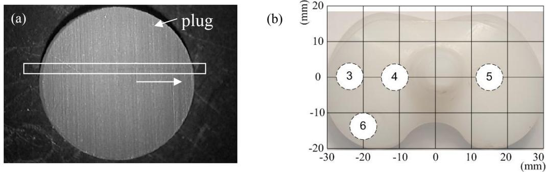
Fig.1. (a) Optical image of a plug prepared with a series of microscratches from left to right and (b) locations of the four plugs 3,4,5,6 in the backside of the UHMWPE tibial insert.
