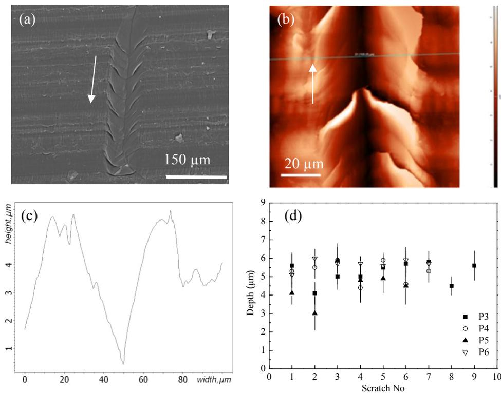
Fig.2. (a) SEM image of a micro-scratch in a UHMWPE plug, (b) AFM image of a partial micro-scratch, (c) Representative cross-section profiles of a micro-scratch and (d) Depth of the micro-scratch on each plug before simulation experiment.
