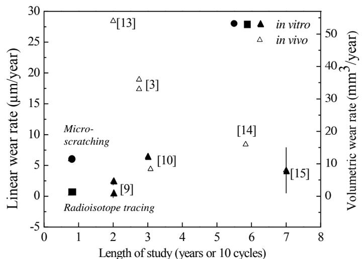
Fig.4. Comparison of the present micro-scratching result at  $1 \times 10^6$  cycles (●) with the result based on a radioisotope tracing study (■) [11,12] and other literature values (▲ of the backside wear rate of tibial inserts in knee prostheses).
