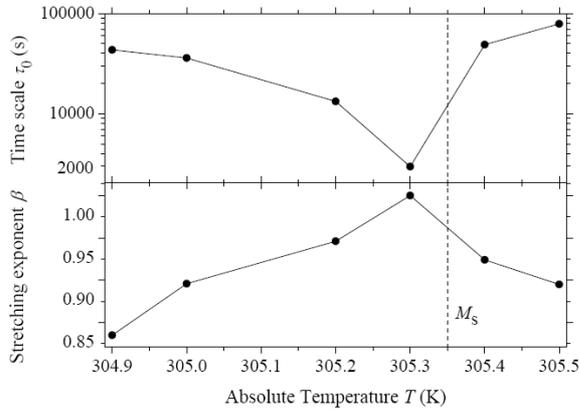
Fig. 4. Results for the characteristic time,  $\tau_0$ , and the stretching exponent,  $\beta$ , at various temperatures near  $M_s$ , determined from data fits using the one-time correlation function.
