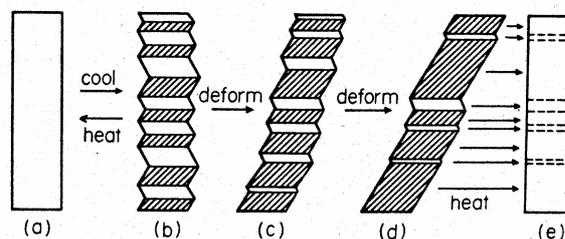
Fig. 1. Illustration of the mechanism for the shape memory effect (after Otsuka *et al.* [2])
