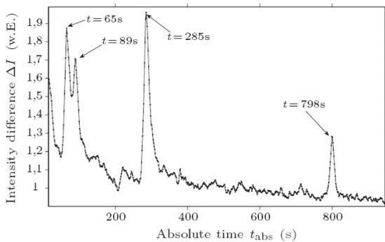
Fig. 6. Sequential intensity differences for averages over 20 exposures, for the data analysed in Fig. 5, as a function of absolute time.
