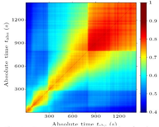
Fig. 5. Two-time correlation function for data recorded at 305.3 K, calculated for a circular region around the maximum of the Bragg reflection.
