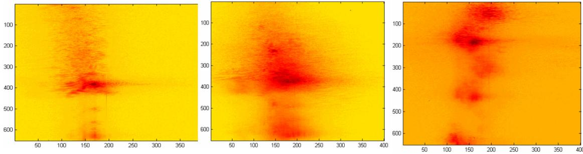
Fig. 3. Images of summed CCD exposures for the (001) Bragg reflection from the  $\text{Au}_{50.5}\text{Cd}_{49.5}$  single crystal at 360 K, (left), 305.5 K (centre) and 270 K (right).
