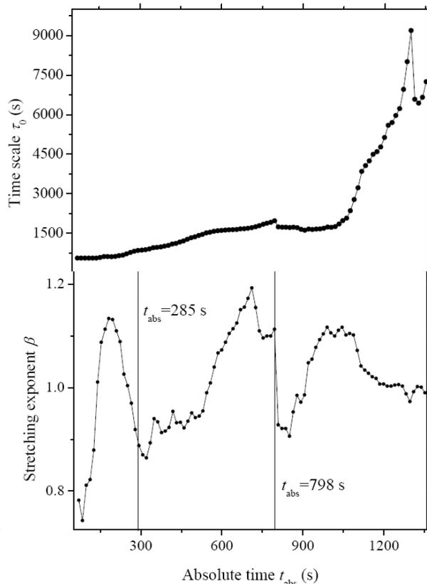
Fig. 7. Characteristic time,  $\tau_0$ , and stretching exponent,  $\beta$ , extracted from the two-time correlation function at 305.3 K
