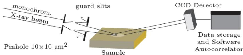
Fig. 2. Schematic setup for x-ray photon correlation spectroscopy measurements.
