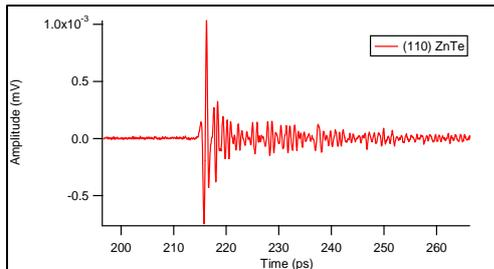
Figure 3. THz time domain signal for (110) ZnTe.
