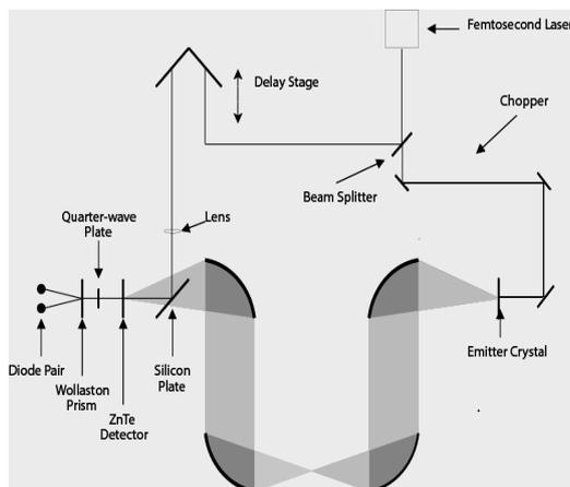
Figure 2. Corresponding block diagram of THz TDS system.
