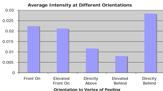
Fig. 4. Average intensity of visible radiation emitted by the adhesive tape for various orientations of the light sensor relative to the line of peeling of the tape. The average frequency of spool rotation for these measurements is 6.0 Hz.
