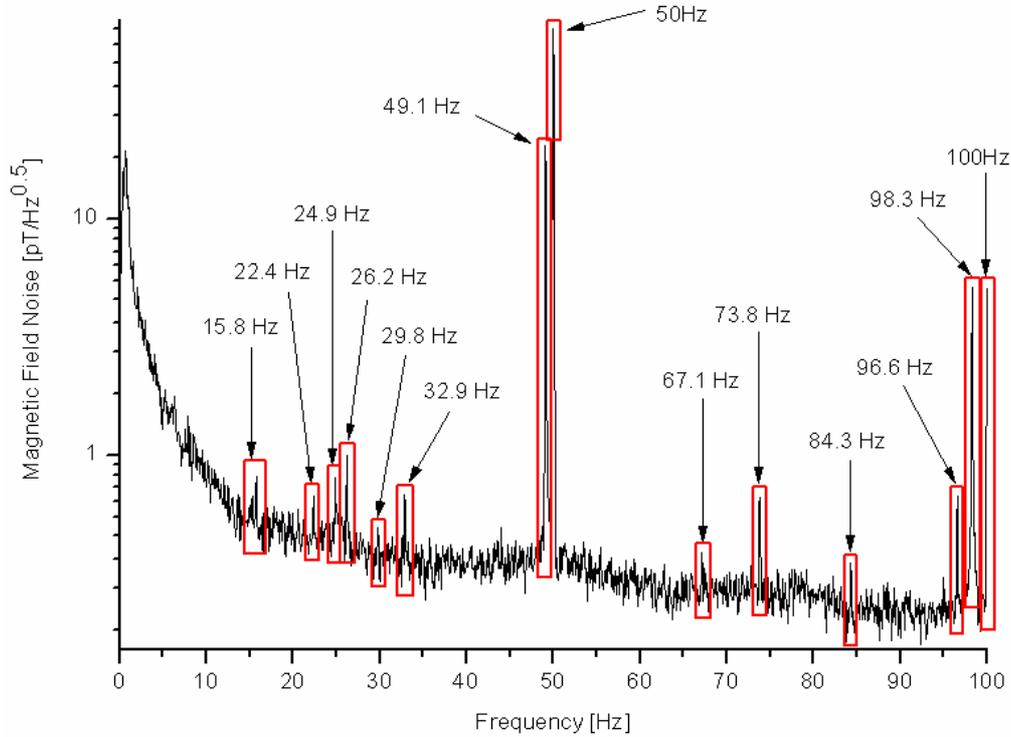
**Fig 2. Peak resonant frequencies when the cryocooler and pumps are operating, with no AV.**
