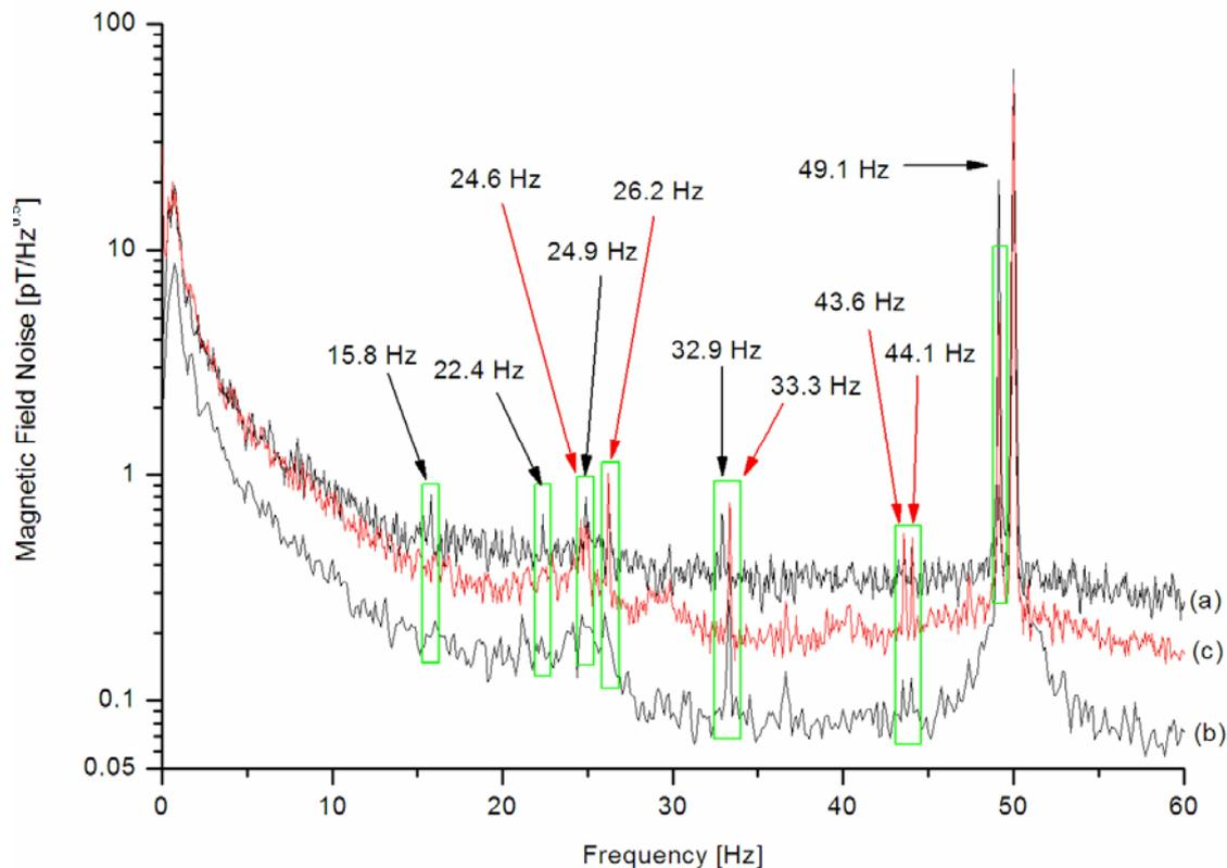
**Fig 3. Comparison of anti-vibration techniques used in conjunction with shielding. (a) only three layers of mu-metal shielding (b) clamping of cryocooler gas lines (c) clamping of cryocooler gas lines and spring support.**
