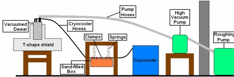
Fig 1. Setup of cryocooled SQUID in the three layered T-shape mu-metal shield, with anti-vibration methods.
