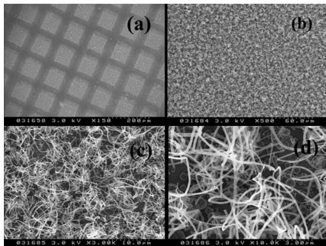
Fig. 2 The morphology of the as-grown CNT deposit. (a): CNT pattern after TEM grid was lifted off. (b-d): larger magnification of as-grown CNTs.
