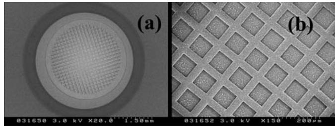
Fig. 1: TEM grid with CNT coating. The TEM grid defined the deposition of CNTs, which are only formed at each square area. (b) high-magnification image of the grid (a).
