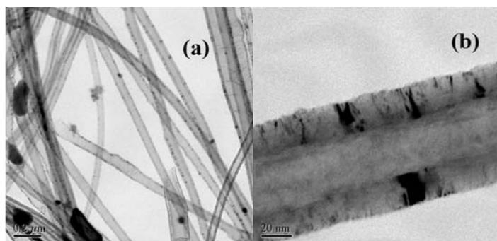
Fig. 3: TEM images showing multi-walled cylindrical structures of CNTs.
