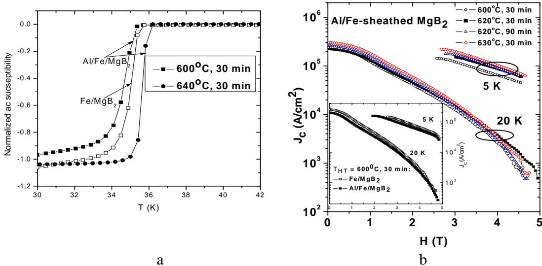
Fig.1. a) Transition temperature of  $Fe/MgB_2$  samples with and without Al; b) critical current density of  $Al/Fe/MgB_2$  samples. Insert is comparison of  $J_c$  for Fe-barrier  $MgB_2$  samples with and without Al
