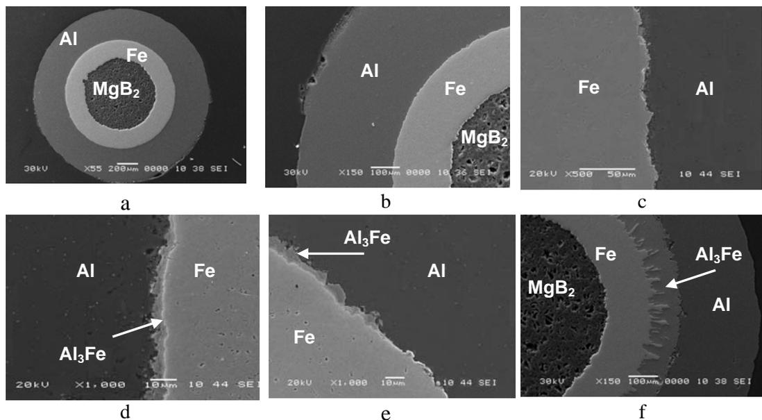
Fig 2. SEM image of the interfaces between Fe and Al sheath for for the Al/Fe/MgB<sub>2</sub> wire a) as drawn and sintered at 600°C for 180 min (b), 620°C for 30 min (c), 620°C for 90 min (d), 640°C for 30 min (e) and 650°C for 30 min (f)
