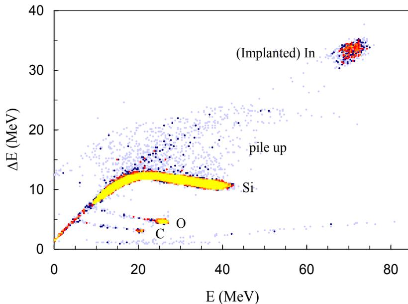
Fig.3: A two-dimensional spectrum from the ERD analysis of silicon wafers implanted with InO<sub>x</sub>. The labels indicate groups of events associated with a specific element. In the colour scale yellow represents the highest number of counts, whereas light-blue corresponds to the lowest number of counts.
