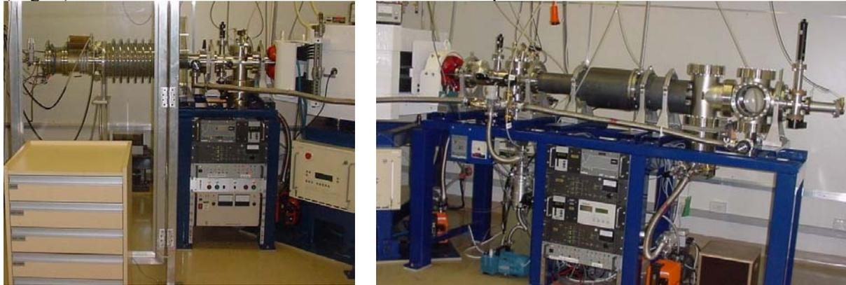
Fig 1: The low energy 150 keV radioactive negative-ion implanter.
