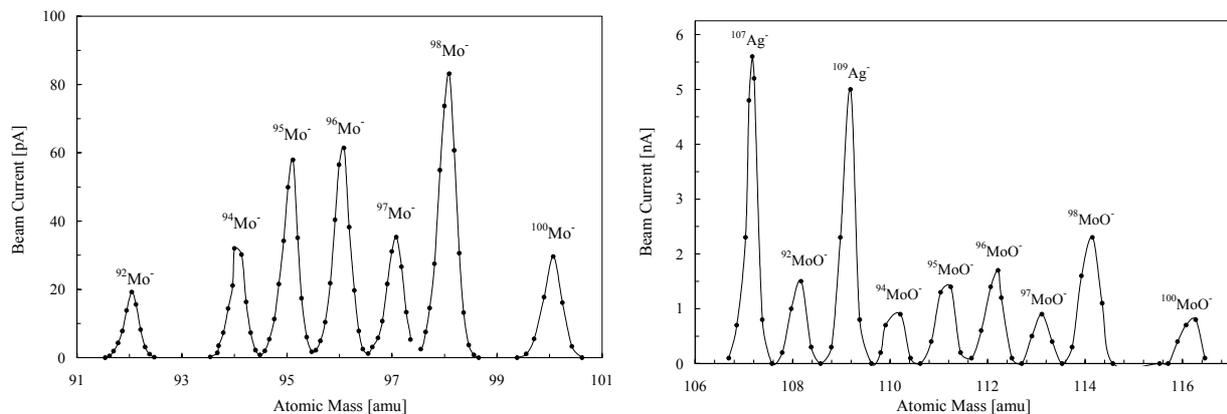
Fig.2: Partial mass spectra for  $\text{MoO}$  cathode. (a) Peaks corresponding to different Mo isotopes can be clearly identified and are well separated. (b) The oxides of these isotopes and two peaks corresponding to residual Ag in the source are also well resolved
